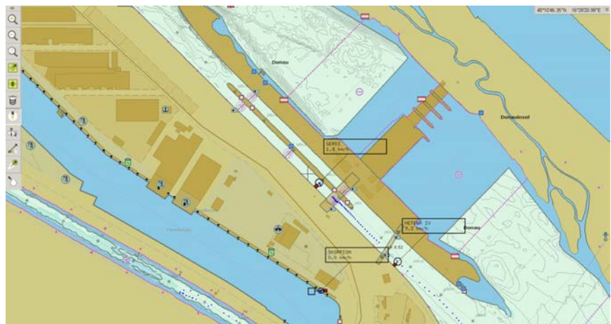
Visualisation of vessel traffic in the immediate proximity of a lock on the Electronic Navigational Chart
