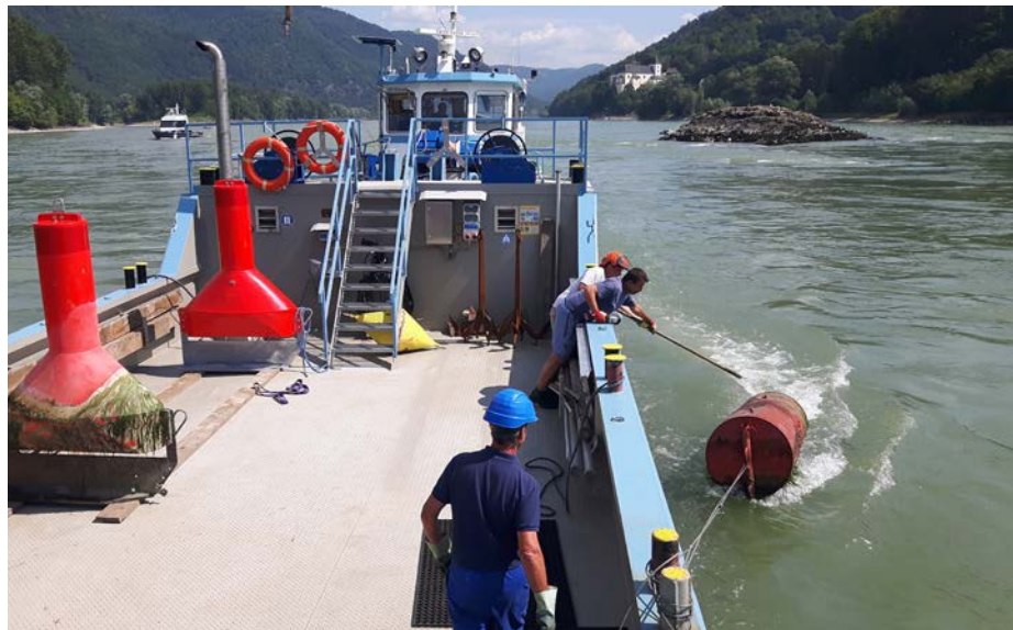
Manipulation of a red buoy to indicate the right-hand limit of the fairway on the Austrian section of the Danube
