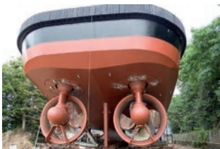
Twin-screw propulsion with ducted propellers
