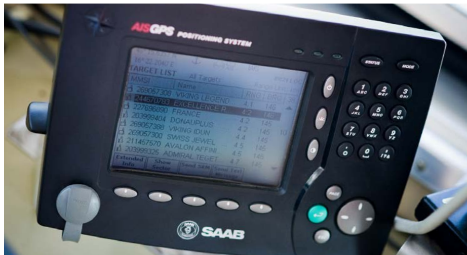
AIS transponder on board an inland vessel
