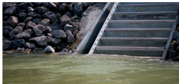
Gauge staff at a gauging site; sample water level at gauge: 95 cm
