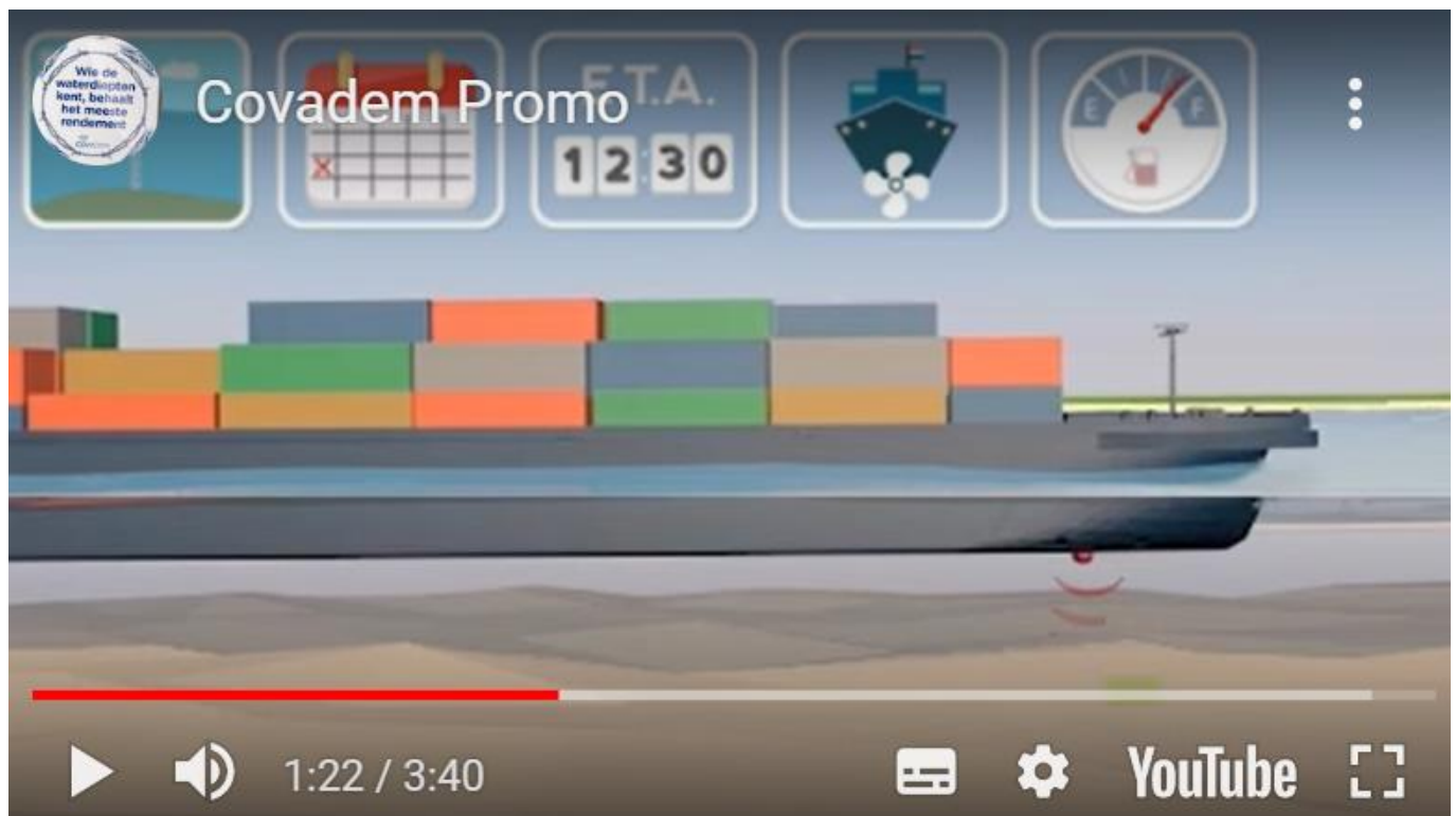
Figure 39: Collective collection of water depth information by commercial vessels operating within the CoVadem initiative, promotion video. IN the front of the vessel, the echo-sounder is located sensing the river bottom. Source: autena 19
