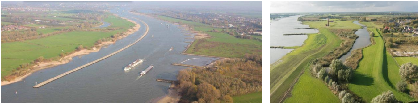
Figure 47: Longitudinal dams (left). Reconnecting flood plains (right). Source: Schielen (2022).
