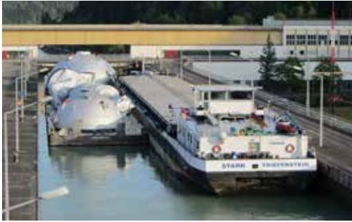
Heavy transport of reactor components, Aschach lock. © viadonau
