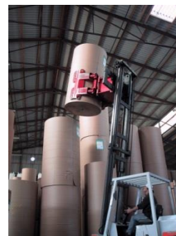
Figure 39: Forklift with paper roll clamps 94
