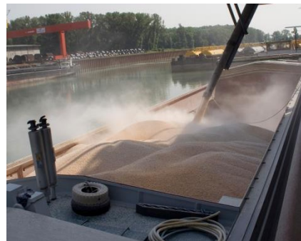
Figure 55: Soybean handling with pump 145
