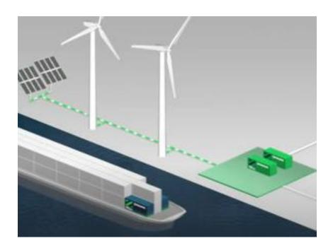
ZESpack charging stations are connected to the electricity grid, so they can be used to stabilize the grid or meet temporary local demand for power.
