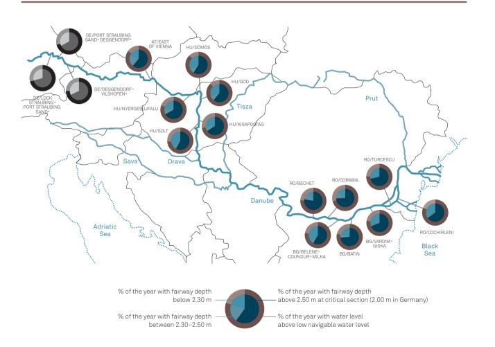
\* In the free flowing section between Straubing and Vilshofen a fairway depth of 2.50 m ist neither developable nor maintanable. In this section the objective is to maintain the fairway depth of 2.00 m related to Low Navigable Water Level. Depicted values in Germany therefore refer to 2.00 m fairway depth.
