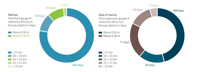
\* Based on the fairway width required for a four-unit pushed convoy travelling downstream without encountering other vessels. Fairway width depends on the river bend radii involved
